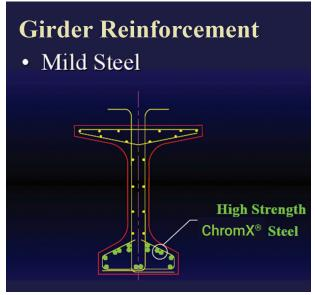
**Daggett Road Bridge over Burns Cut-off, Stockton, CA**Bridge girders constructed with ChromX<sup>®</sup> (100ksi design).
