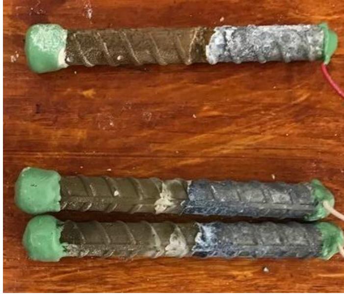
Figure 3.21: Rapid Macrocell Test. Specimen A1094-4 anode bar (top) and cathode bars (bottom)
