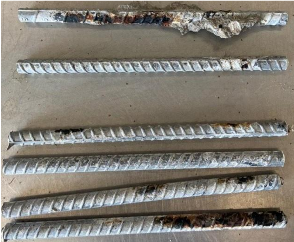
Figure 3.60: Southern Exposure test. Specimen A1094-4 after 96 weeks of testing. Top mat (top) and bottom mat (bottom).
