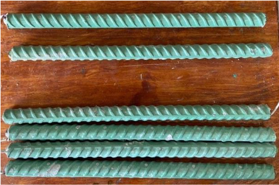
Figure 3.44: Southern Exposure test. Specimen ECR-2 after 96 weeks of testing. Top mat (top) and bottom mat (bottom).
