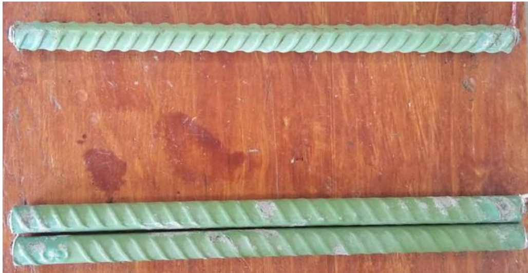
Figure 3.56: Cracked beam test. Specimen ECR-UV-1000-ND-1 after 96 weeks of testing. Top mat (top) and bottom mat (bottom).
