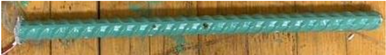
Figure 3.50: Top bar of cracked beam test. Specimen ECR-ND-1 after 96 weeks of testing.
