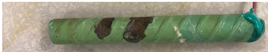
Figure 3.15: Rapid Macrocell Test. Specimen ECR-UV-1000-4 anode bar after disbondment test
