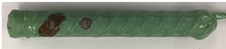
Figure 3.13: Rapid Macrocell Test. Specimen ECR-2 anode bar after disbondment test
