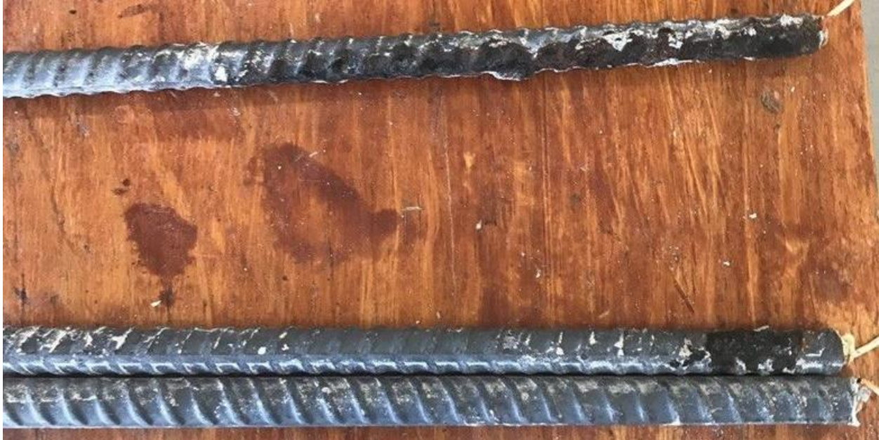
Figure 3.68: Cracked beam test. Specimen A1035-Ipanex-6 after 96 weeks of testing. Top mat (top) and bottom mat (bottom).
