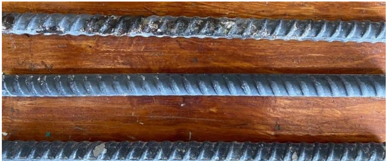
Figure 3.67: Cracked beam test. Specimen A1035-1 after 96 weeks of testing. Top mat (top) and bottom mat (bottom).
