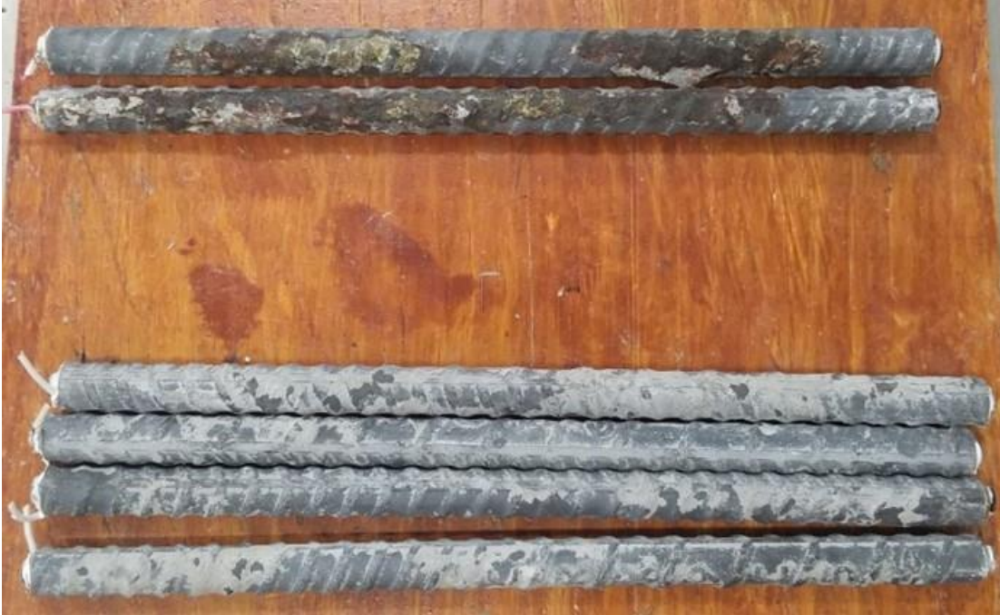
Figure 3.64: Southern Exposure test. Specimen A1035-5 after 96 weeks of testing. Top mat (top) and bottom mat (bottom).
