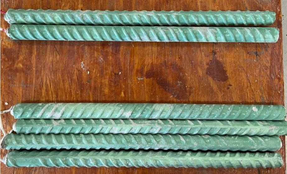
Figure 3.46: Southern Exposure test. Specimen ECR-ND-2 after 96 weeks of testing. Top mat (top) and bottom mat (bottom).
