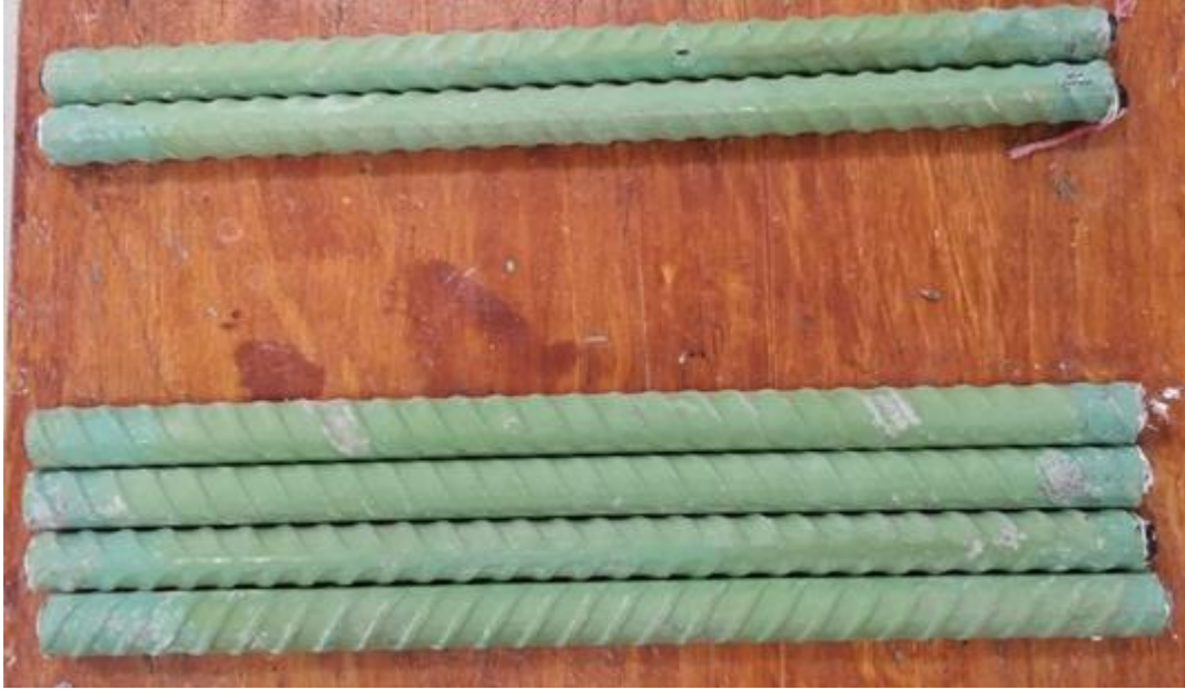
Figure 3.53: Southern Exposure test. Specimen ECR-UV-1000-ND-1 after 96 weeks of testing. Top mat (top) and bottom mat (bottom).
