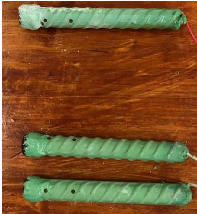
Figure 3.14: Rapid Macrocell Test. Specimen ECR-UV-1000-4 anode bar (top) and cathode bars (bottom)
