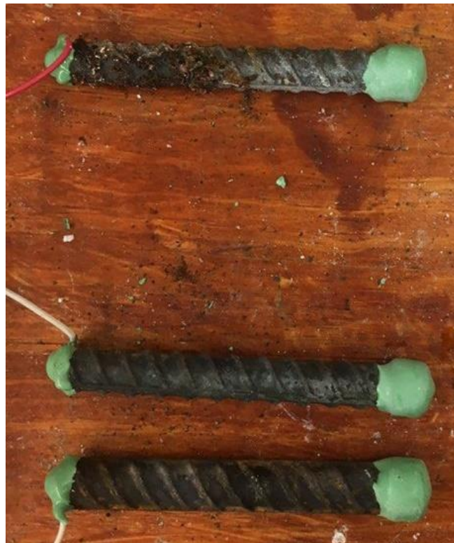
Figure 3.11: Rapid Macrocell Test. Specimen Conv-B-5 anode bar (top) and cathode bars (bottom)
