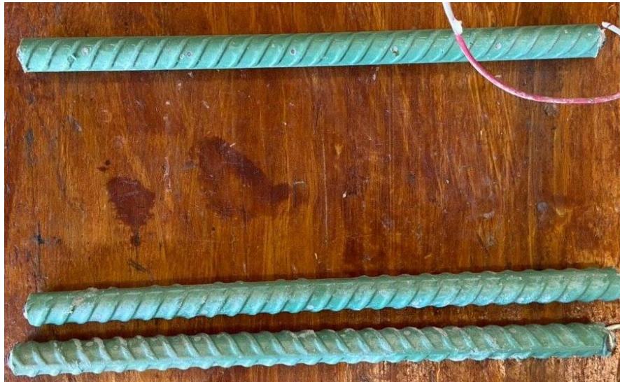
Figure 3.47: Cracked beam test. Specimen ECR-3 after 96 weeks of testing. Top mat (top) and bottom mat (bottom).
