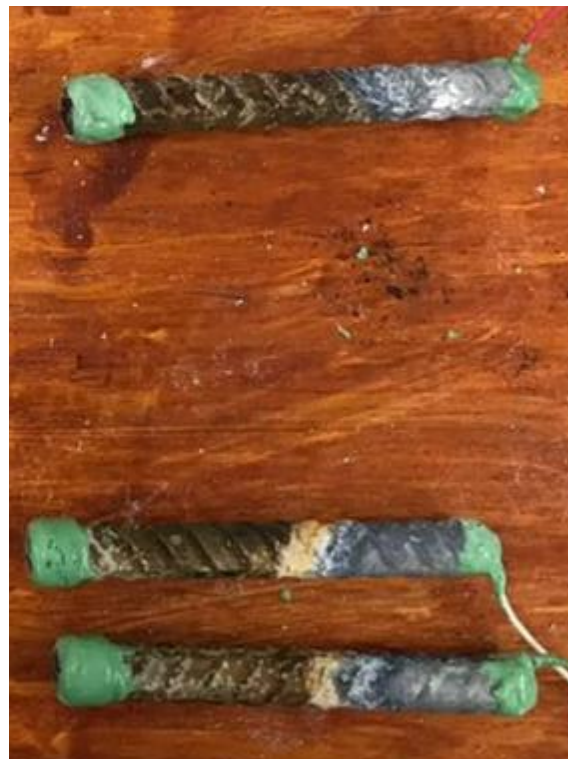
Figure 3.20: Rapid Macrocell Test. Specimen A767-1 anode bar (top) and cathode bars (bottom)
