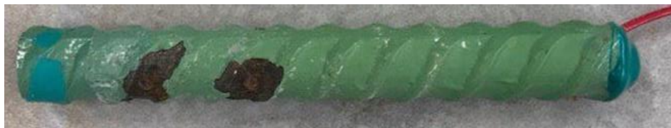
Figure 3.16: Rapid Macrocell Test. Specimen ECR-UV-500-5 anode bar after disbondment test
