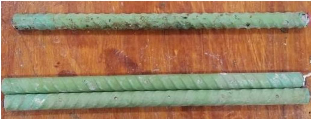
Figure 3.54: Cracked beam test. Specimen ECR-UV-1000-2 after 96 weeks of testing. Top mat (top) and bottom mat (bottom).
