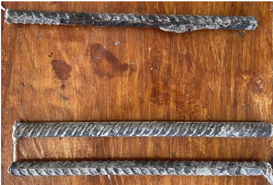
Figure 3.69: Cracked beam test. Specimen A1035-Xypex-2 after 96 weeks of testing. Top mat (top) and bottom mat (bottom).
