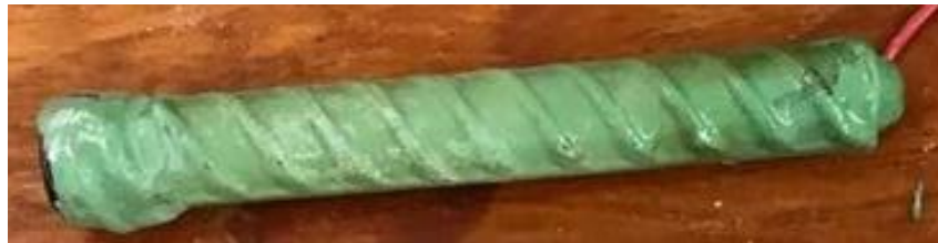
Figure 3.19: Rapid Macrocell Test. Specimen ECR-ND-6 anode bar after disbondment test
