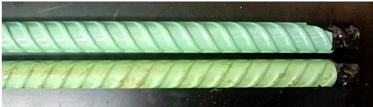
Figure 2.2: ECR before (top) and after (bottom) UV exposure.
