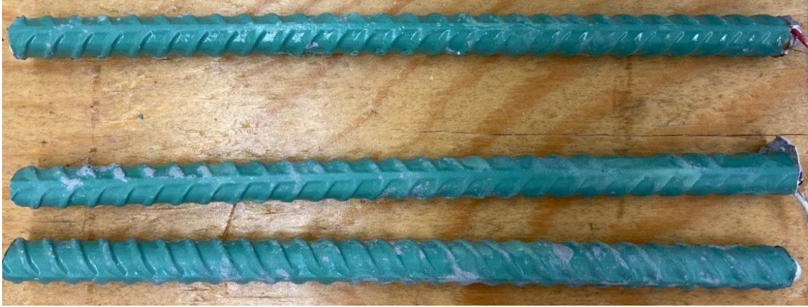
Figure 3.49: Cracked beam test. Specimen ECR-ND-2 after 96 weeks of testing. Top mat (top) and bottom mat (bottom).
