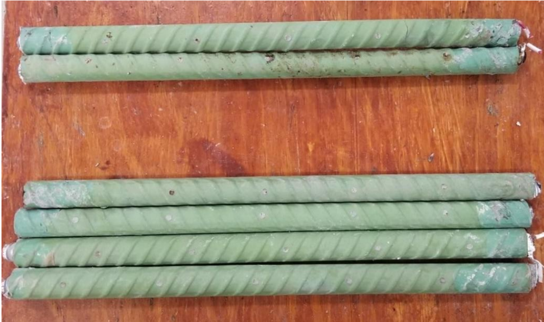
Figure 3.51: Southern Exposure test. Specimen ECR-UV-1000-1 after 96 weeks of testing. Top mat (top) and bottom mat (bottom).
