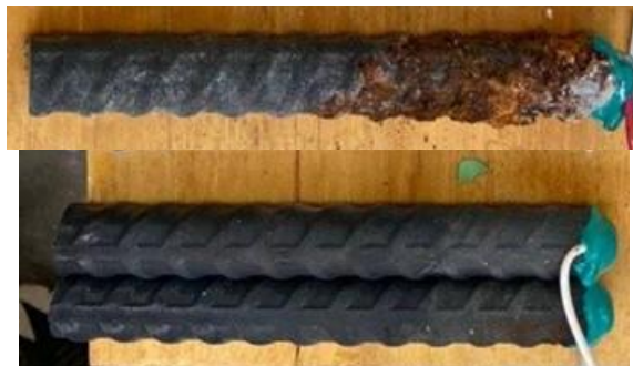
Figure 3.22: Rapid Macrocell Test. Specimen A1035-6 anode bar (top) and cathode bars (bottom)
