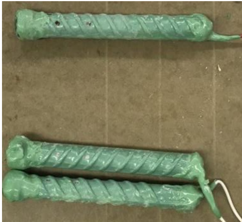
Figure 3.12: Rapid Macrocell Test. Specimen ECR-2 anode bar (top) and cathode bars (bottom)
