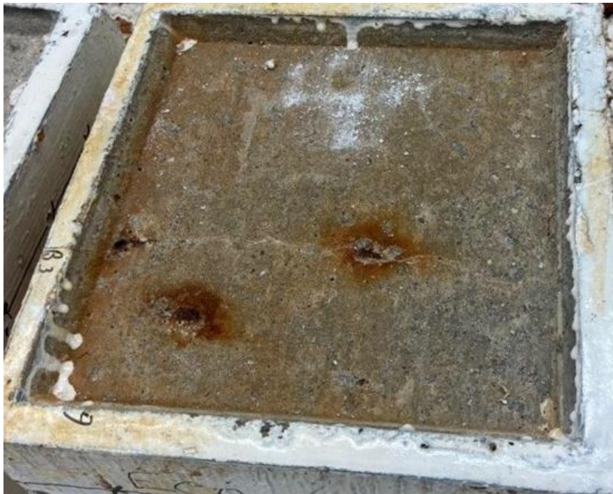
Figure 3.41: Southern Exposure test. Surface staining on specimen with conventional reinforcement.
