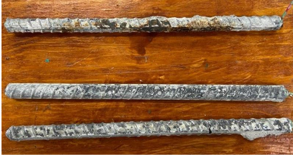
Figure 3.61: Cracked beam test. Specimen A1094-6 after 96 weeks of testing. Top mat (top) and bottom mat (bottom).
