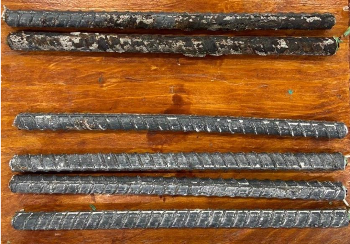
Figure 3.40: Southern Exposure test. Specimen Conv-C-1 after 96 weeks of testing. Top mat (top) and bottom mat (bottom).
