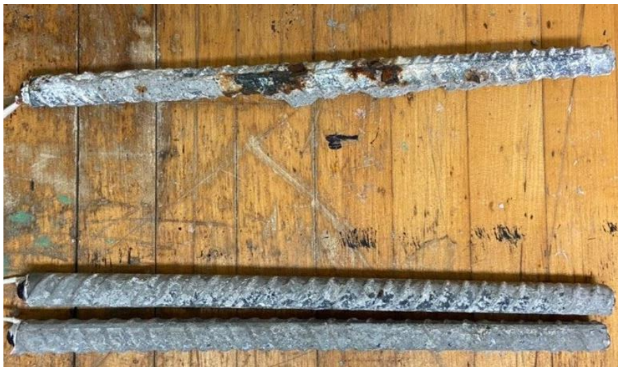
Figure 3.59: Cracked beam test. Specimen A767-3 after 96 weeks of testing. Top mat (top) and bottom mat (bottom).
