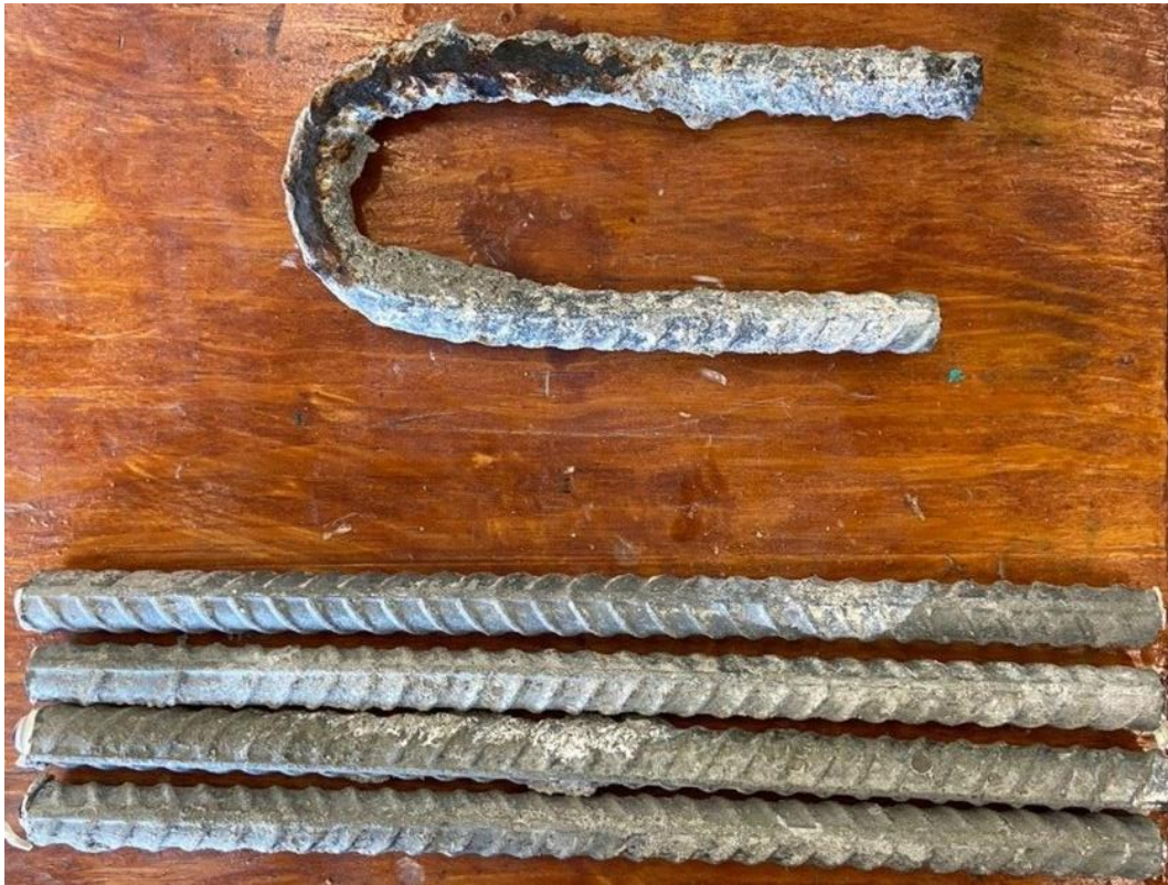
Figure 3.62: Southern Exposure test. Specimen A767-b-2 after 96 weeks of testing. Top mat (top) and bottom mat (bottom).
