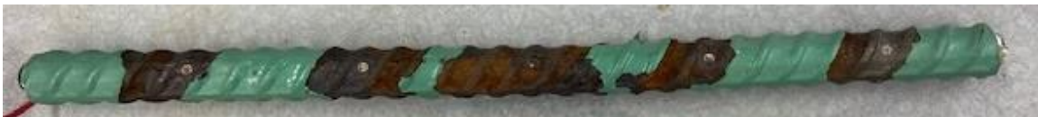
Figure 3.48: Cracked beam test. Top bar of specimen ECR-2 after disbondment test.
