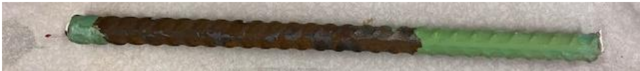
Figure 3.52: Southern Exposure test. Top bar of specimen ECR-UV-1000-1 after disbondment test.
