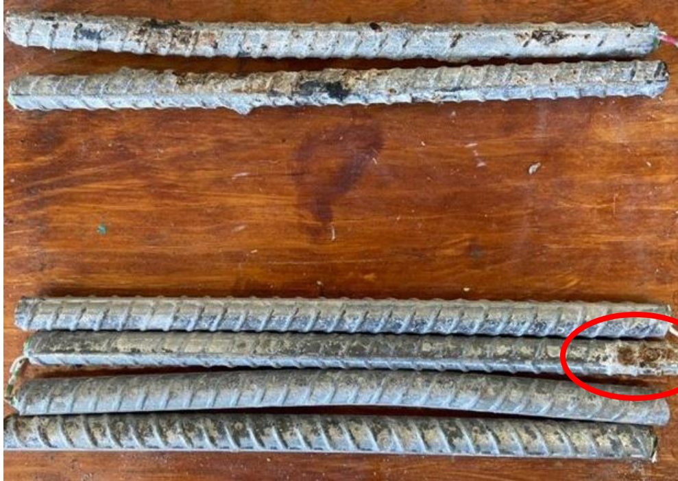
Figure 3.58: Southern Exposure test. Specimen A767-2 after 96 weeks of testing. Top mat (top) and bottom mat (bottom). Corrosion on bottom mat circled.
