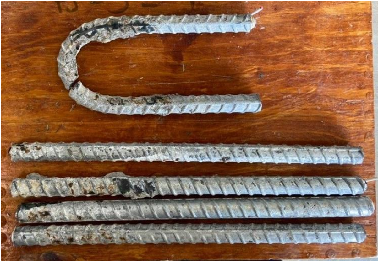
Figure 3.63: Southern Exposure test. Specimen A1094-b-2 after 96 weeks of testing. Top mat (top) and bottom mat (bottom).
