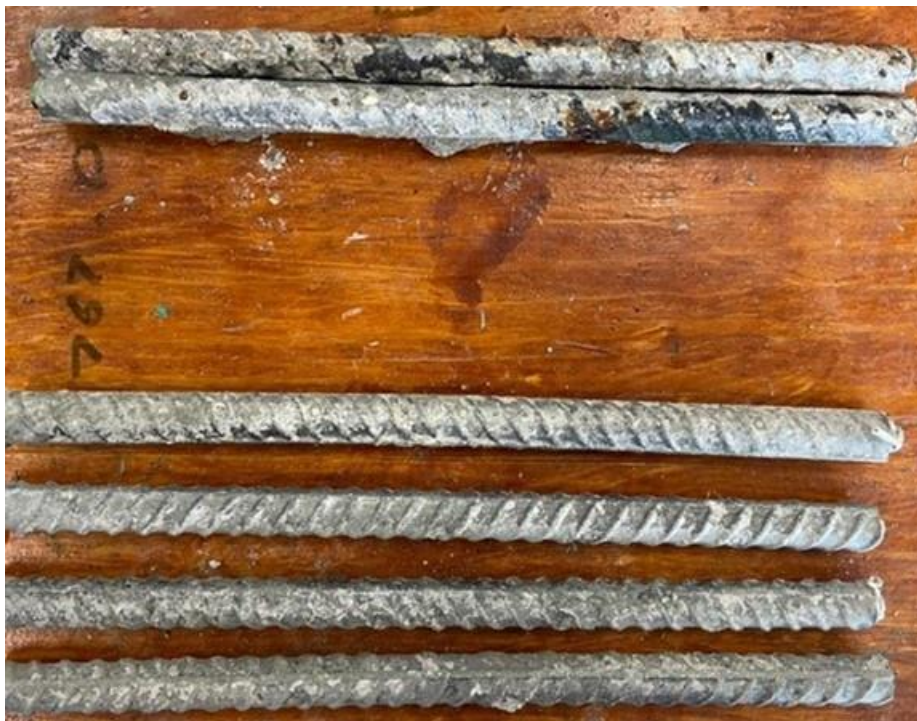
Figure 3.57: Southern Exposure test. Specimen A767-3 after 96 weeks of testing. Top mat (top) and bottom mat (bottom).
